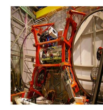
The Fizeau interferometer LINC-NIRVANA [2] of the Large Binocular Telescope (LBT) detects p different images of the same object, corresponding to p different rotations of LBT, in order to get the maximum resolution in all directions.
